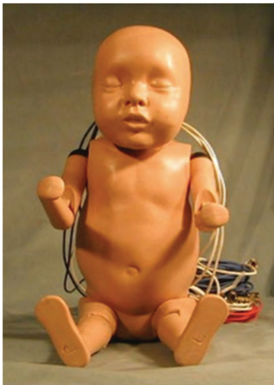
FIG. 1. Aprica 2.5 anthropomorphic test device (ATD). Color image is available online at www.liebertpub.com/neu
