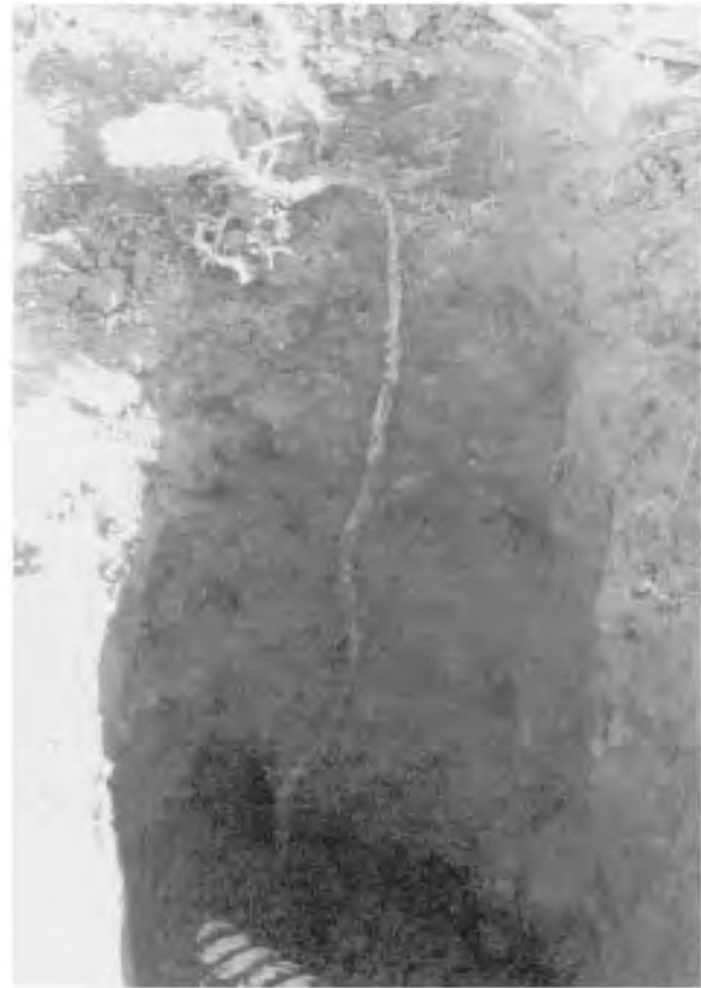
Fig. 4. Earthworm burrow closely associated with the buried tile. This burrow approached within 3 cm of the tile and had an average infiltration rate of 236 \text{ mL min}^{-1} .
